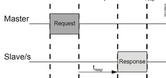
Maximum response time when reading: ..  $t_{resp} = 210$  ms
