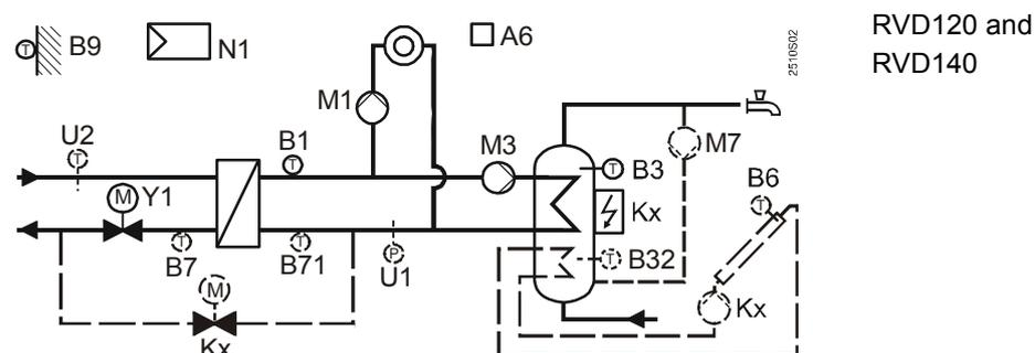
Heating circuit control with d.h.w. heating (storage tank).
