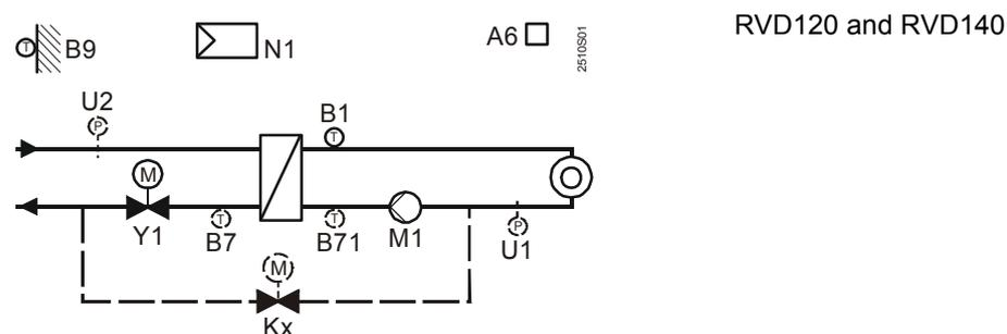
Heating circuit control without d.h.w. heating
