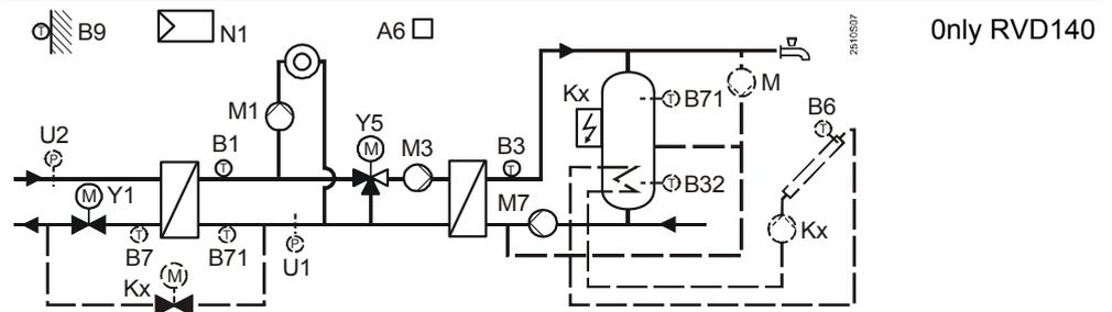
Two heat exchangers connected in series for heating circuit and d.h.w. heating. Instantaneous storage tank connected to the second heat exchanger, with mixing valve control for d.h.w.
