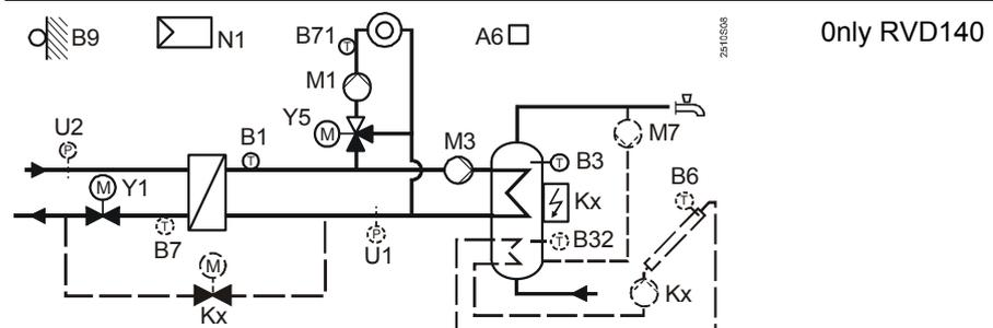
Heating circuit control with d.h.w. heating. Heating circuit with mixing valve, storage tank with charging pump.
