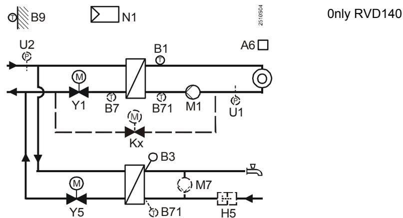
Separate heat exchangers for heating circuit and d.h.w. heating (instantaneous system). Sensor B71 can be used as follows:
