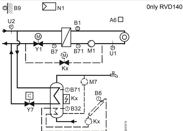
Heat exchanger for the heating circuit, d.h.w. heating via the district heat primary circuit, control of the d.h.w. temperature via an electrothermal actuator. Circulating pump, refill function, electric immersion heater and solar d.h.w. heating optional.
