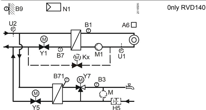
Separate heat exchangers for heating circuit and d.h.w. heating, two-stage d.h.w. control: 1st stage in the primary return, 2nd stage with mixing valve in the secondary flow. Flow switch, refill function and externally controlled circulating pump optional. Selectable idle heat function.
