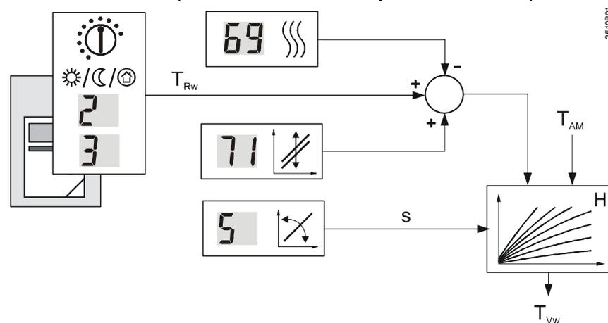
Generation of setpoint with weather-compensated control without room temperature
