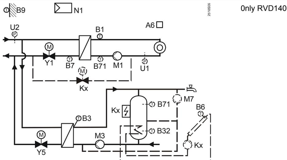
Separate heat exchangers for heating circuit and d.h.w. heating. Instantaneous storage tank connected to separate heat exchanger, d.h.w. charging with charging pump.
