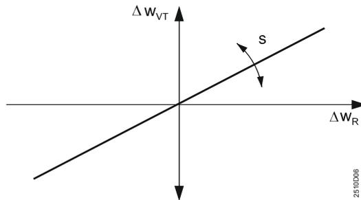
Effect of room temperature setpoint change on the flow temperature setpoint
