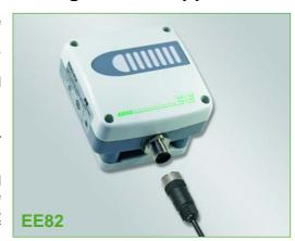
Measuring ranges of 0...2000/5000/7000ppm correspond to an analogue interface of 0 - 5/10V or 4 - 20mA. Selectively a switching output with adjustable switching point and hysteresis is available.
